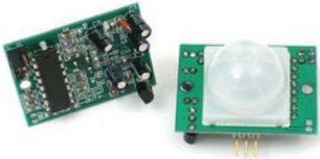
So a PIR or "passive infra red" is a sensor that detects changes in infra red light. So do you remember that box in the top corner of the rooms in your house? It's a PIR! A PIR use the range of light that us humans can't see, but this little device can. When it detects changes in the infra red light E.G. When someone walk in front of it, it tells what it's connected to that something has happened.
